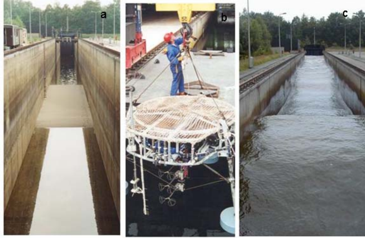
Figure 1. (a) Photograph of the Deltaflume showing the sand bed at approximately midway along the flume and the wave generator at the far end of the flume. (b) The instrumented tripod platform, STABLE, used to make the measurements. (c) A surface wave propagating along the flume.
